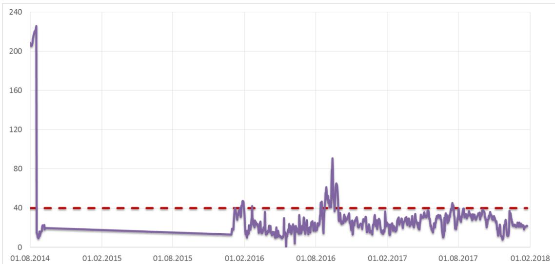
Figure C.1.20 – Global Average Time Transfer Error based on a measurement interval of 24 hours
