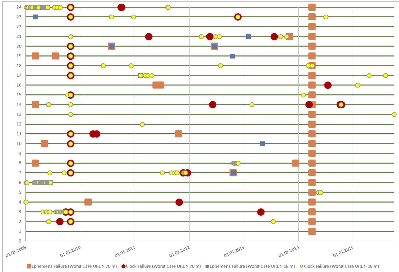
Figure C.2.1 – 2009–2015 GLONASS Failures (for every satellite of the 24–sat constellation)
