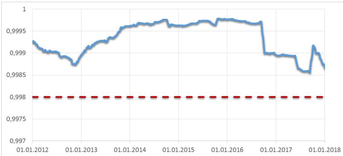
Figure C.1.9 — CSA SIS Continuity during one hour, averaged over the constellation, based on measurement interval of 1 year without prior notice
