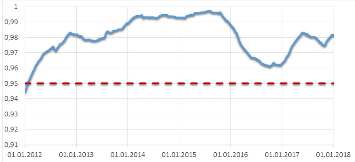
Figure C.1.10 — CSA SIS Per-slot Availability (an average over all slots in the constellation, based on measurement interval of 1 year)
